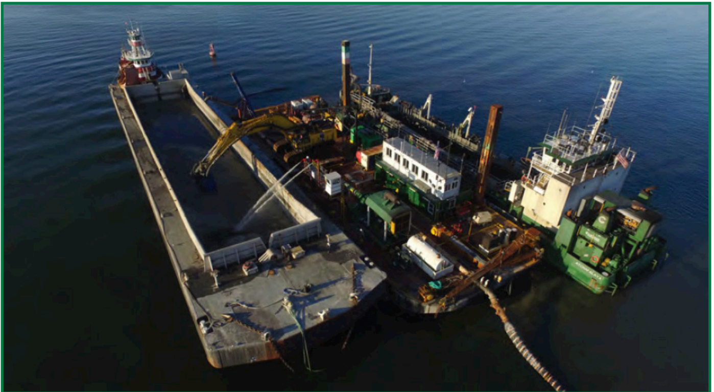
The Kraken offloading one of the Cashman large hopper barges and preparing to assist the TSHD Atchafalaya to pump out to a CDF.
